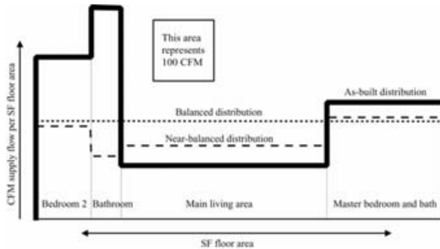
Figure 3-14 Graphical representation of ADS balancing, single section home
