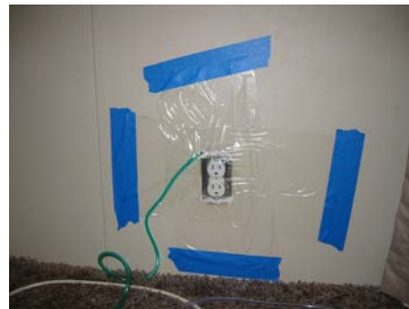
Figure 2-6 Pressure probe in wall
