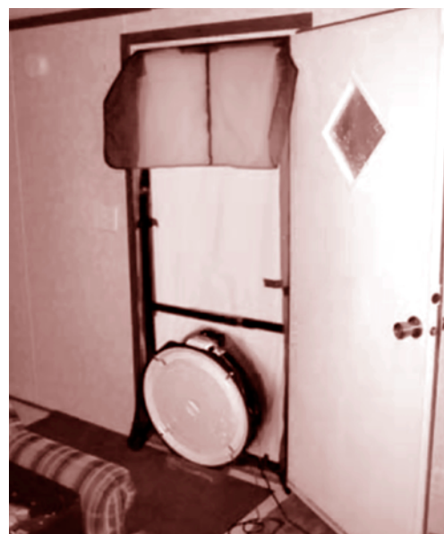
Blower door test measures air infiltration.
