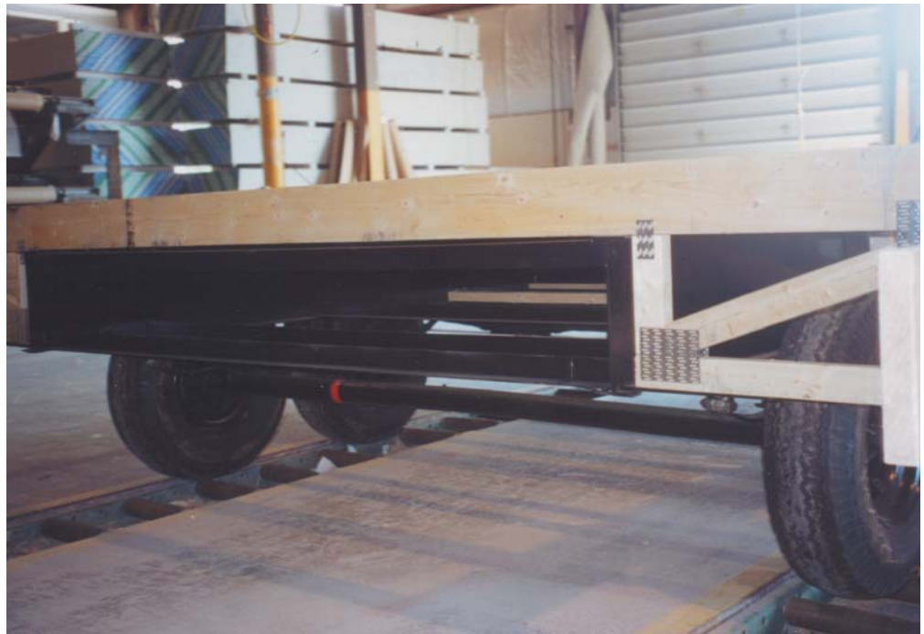
The removable wheel assemblies support a pair of longitudinal steel beams under the house and are used to transport the home to the site.
